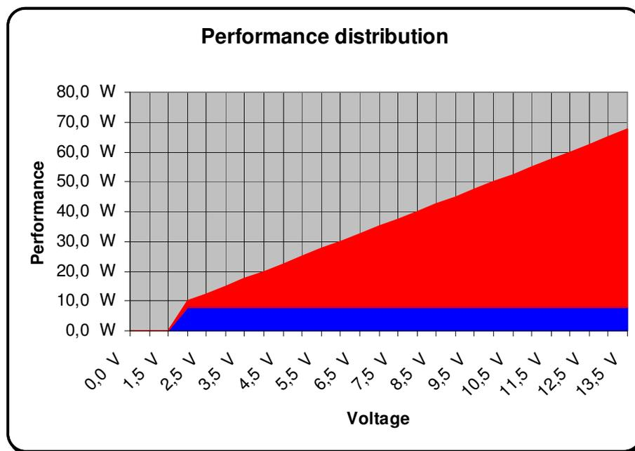
This figure shows that 8 Watts is used for gas production at each voltage if we fix amperage. Blue area shows how much energy can be used for gas production, red area shows how much energy heats our device. (A note for experts: This is an assumption, if you use the same electrolyte amount and you measures your system's amperage you will find that its absolutely different to this diagram.) Finally this diagram shows that most significant part of the energy will produce heat in case of 13 Volts.
